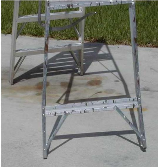
Figure 6: Type II Racking failure.
