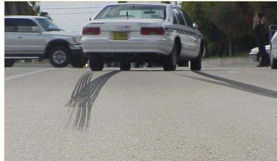
Figure 1. Typical locked-wheel skid marks.
