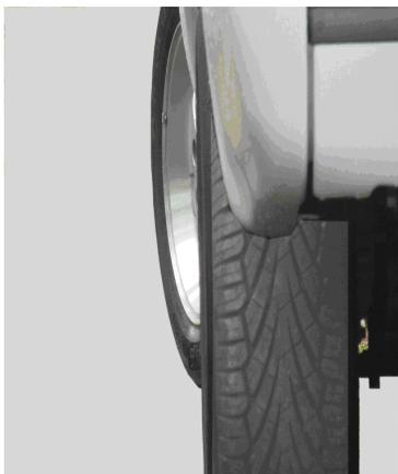
**Figure 9: Front and rear tires are not parallel during steer maneuver (view from rear).**
