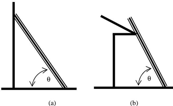
Figure 1: Straight ladder mounting.
