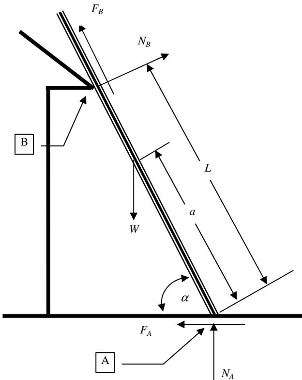
Figure 2: Free Body diagram of a ladder leaning on edge.
