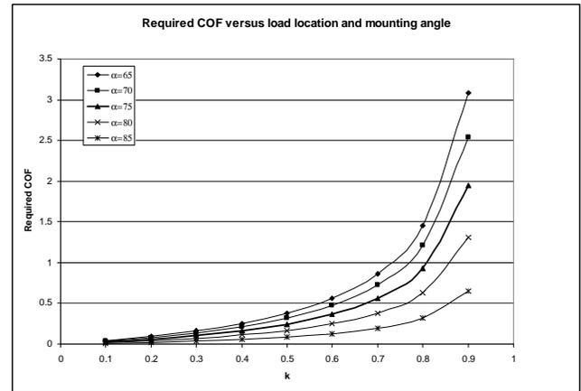
Figure 3: Required COF at point A to avoid slippage.
